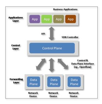
Figure 1. Software-Defined Network Architecture
