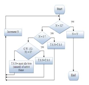
Fig. 8. De- compression process
