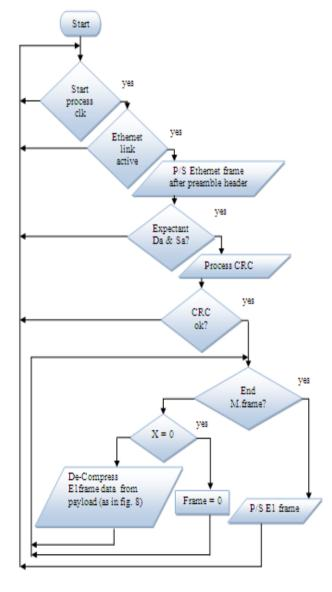
Fig. 6. G.W. RX at Active M. frame mode
