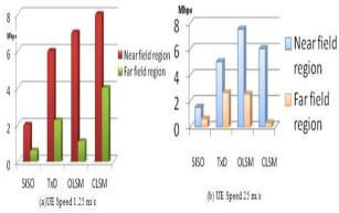
Figure 7. Throughput with Changed Speed for Transmission Modes
