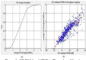
Figure 4. UE Wideband SINR to Throughput Mapping
