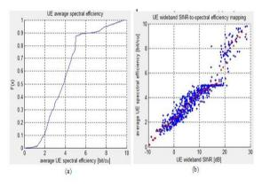
Figure 5. UE Wideband SINR to Spectral Efficiency Mapping
