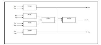
Figure 2: Block Diagram of 2 bit Karatsuba Multiplier for polynomial multiplication
