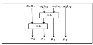
Figure 1: Block Diagram of 2 bit Array Multiplier
